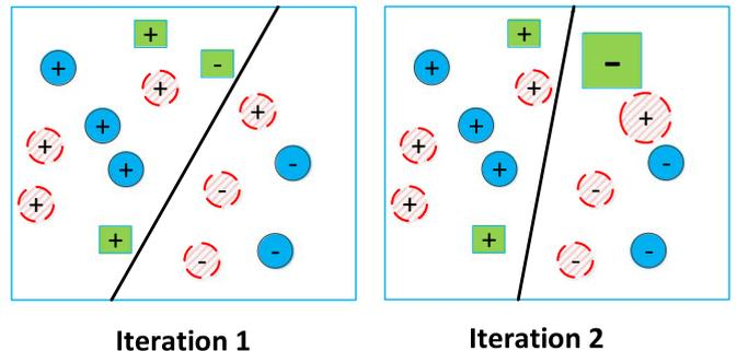
Fig. 3. An example of the EL phase of *HYDRA*. We have instances from two source projects (the blue and red circles), and instances from a training target data (the squares). “+” and “-” represent clean and defective labels respectively. The solid lines in the figures represent how the classifiers predict clean and defective instances.
